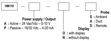
**Example : HM110 – ANS** Ambient humidity transmitter HM110, active 0-10 V, without display
